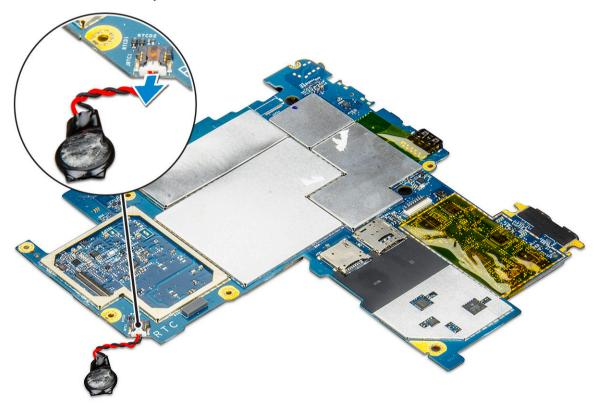
NOTE: If you can easily disconnect the coin cell battery cable from beneath the connector on the system board, you need not remove the system board to remove the coin cell battery.
