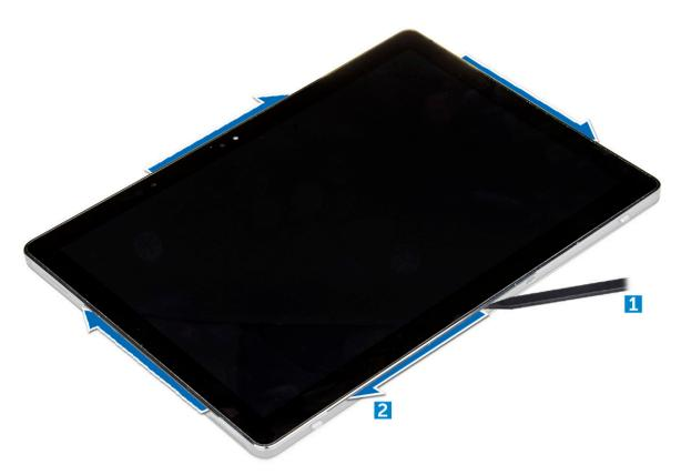
7 Flip the display panel on a plane surface .
