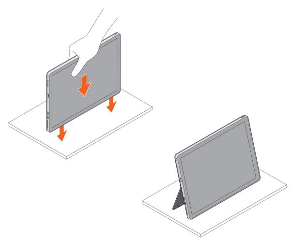
ONOTE: The pegs at the bottom of the tablet allow the kickstand to open.
