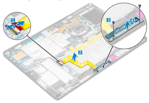
Lift the docking board after releasing the cable from the adhesive.
