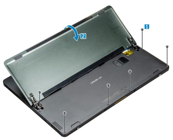
6 Use a plastic scribe [1] to pry the edges [2] of the display panel starting from the bottom side first (near the docking port).
