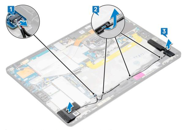
c Remove the speaker cable from the connector on the system board [].
