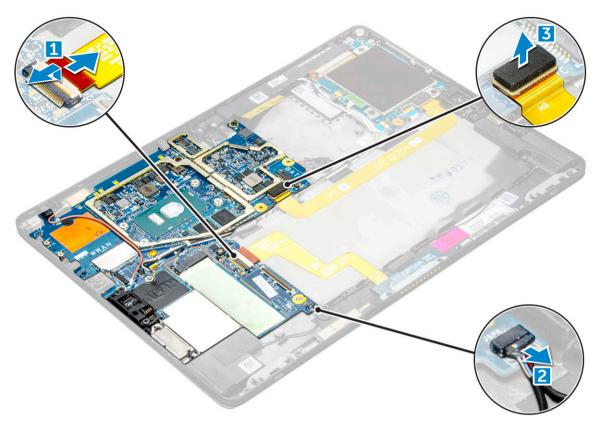
Un route the antenna cables from the routing clips [1,2, 3, 4].
